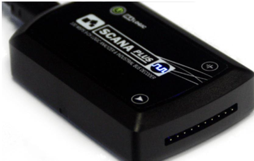
Figure 16: ScanaPLUS logic analyzer device
