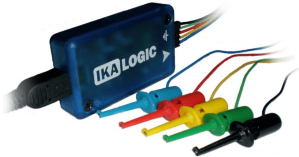
Figure 19: scanalogic-2 logic analyzer
